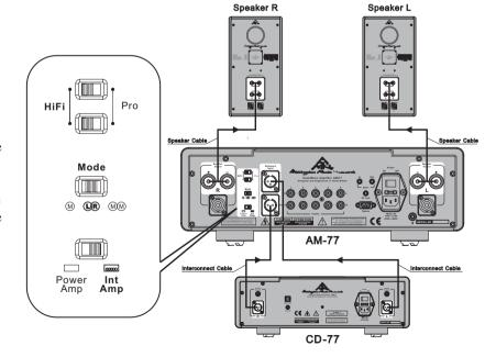
Figure 1.3 - System connection using banana plug/spade connector equipped speaker cables
